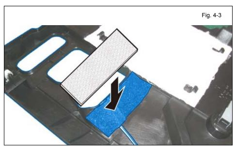
d. Apply 1 Foam Tape to the GBS Microphone as shown.
