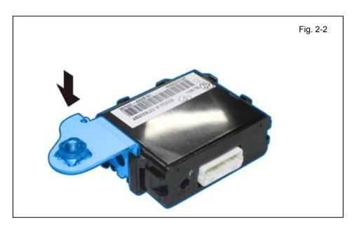
b. Attach the GBS ECU Bracket to the GBS ECU as shown.
